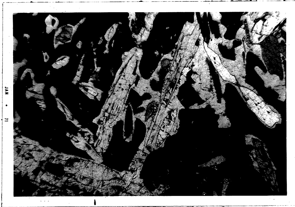
Fig. 8; Relationship between hercynite and anthophyllite showing corrosion edges and interstitial cordierite. Sample FM-1- (X-Nicols; X 25).
