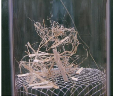
Fig. 3.10. Test of the 3 g random hemp mixture at the predetermined terminal velocity.
