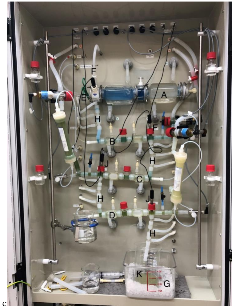
Figure 1. Labelled photo of the TNO gastro-intestinal model (TIM-1) A: gastric compartment B: duodenal compartment C: jejunal compartment D: ileal compartment E: gastric secretion pumps F: pH electrode G: water bath H: peristaltic valve pump I: duodenal secretion pump J: pH electrode K: collecting vessel for ileal delivery
