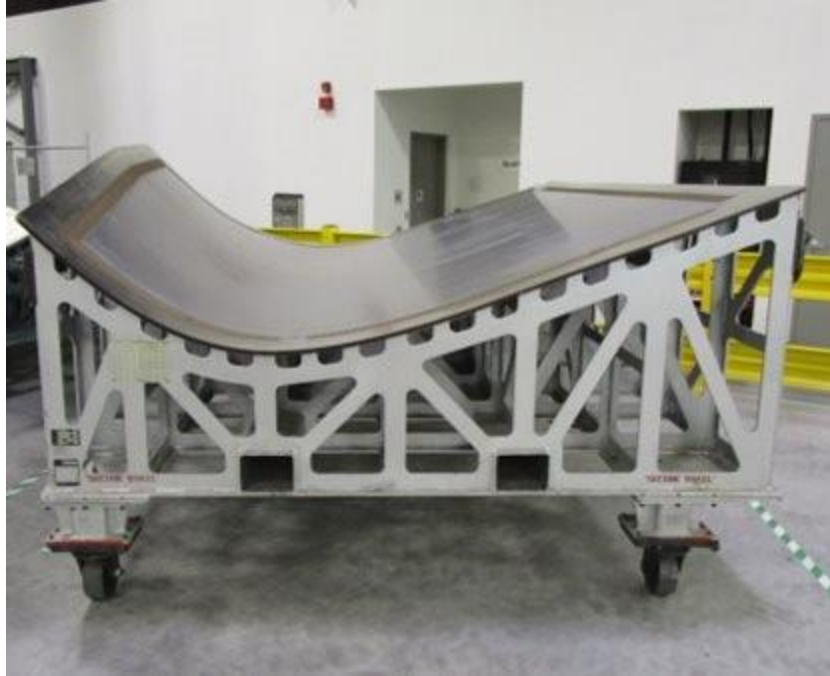
Figure 1: A Layup Mandrel (LM), used with permission [2]
