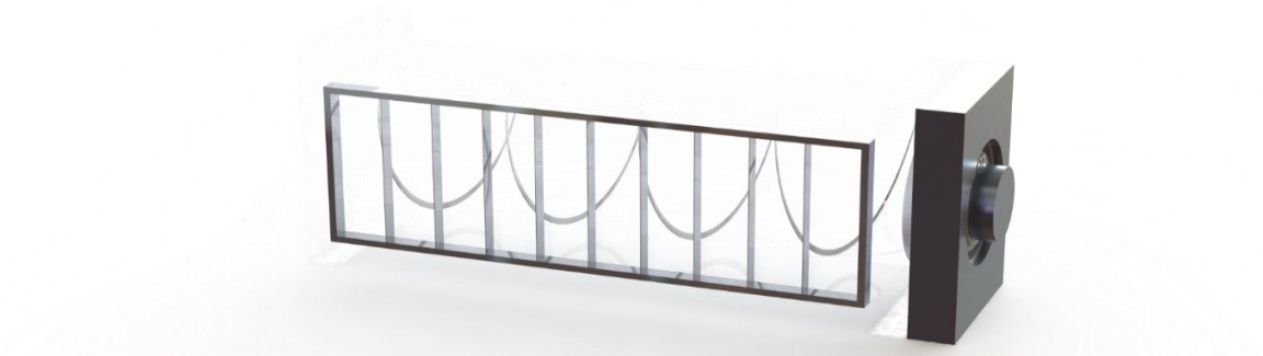
Figure B - 40: Sinusoid device with aluminum embed grids and aluminum bearing casing.
