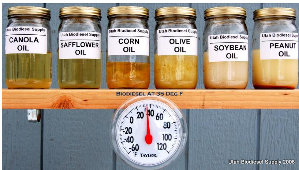
Figure 1.4: Different levels of crystallization of biodiesel from various feedstock at the same temperature of 1.67^{\circ}\text{C} [11].
