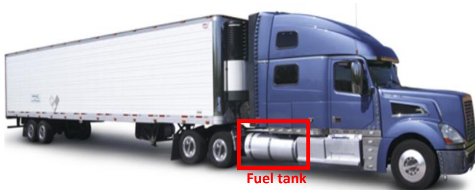
Figure 1.5: Diesel tractor-trailer truck to operate with B100 in winter. The goal is to retrofit the existing fuel tanks with a PCM heated system so that there is limited change to the configuration and operation of the truck. Image source: [26].
