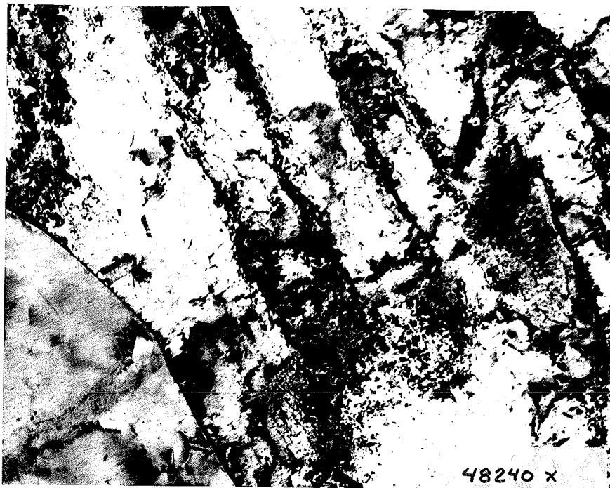
Figure 4.21(b): Dislocation Structures Resulting From a 13.5% Reduction in Area (Metal 6)
