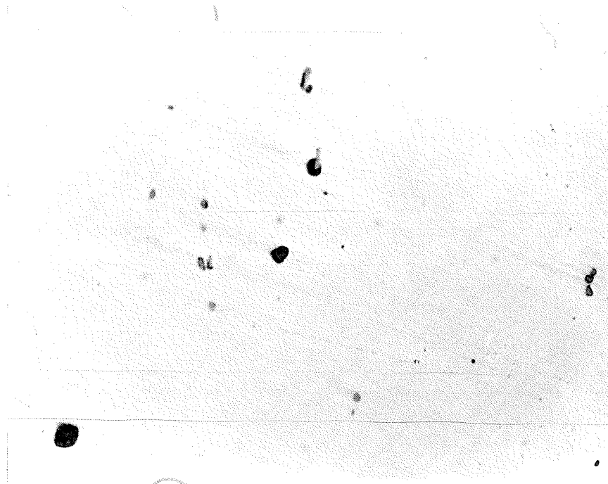
Figure 4.3(b): Inclusion Distribution in Metal 2, 1000X
