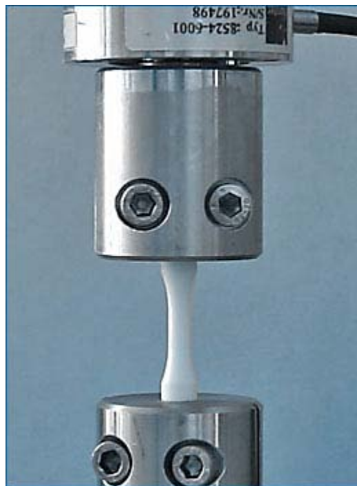
Figure 2.5: Set up of compression test on a dumbbell shape specimen [84].
