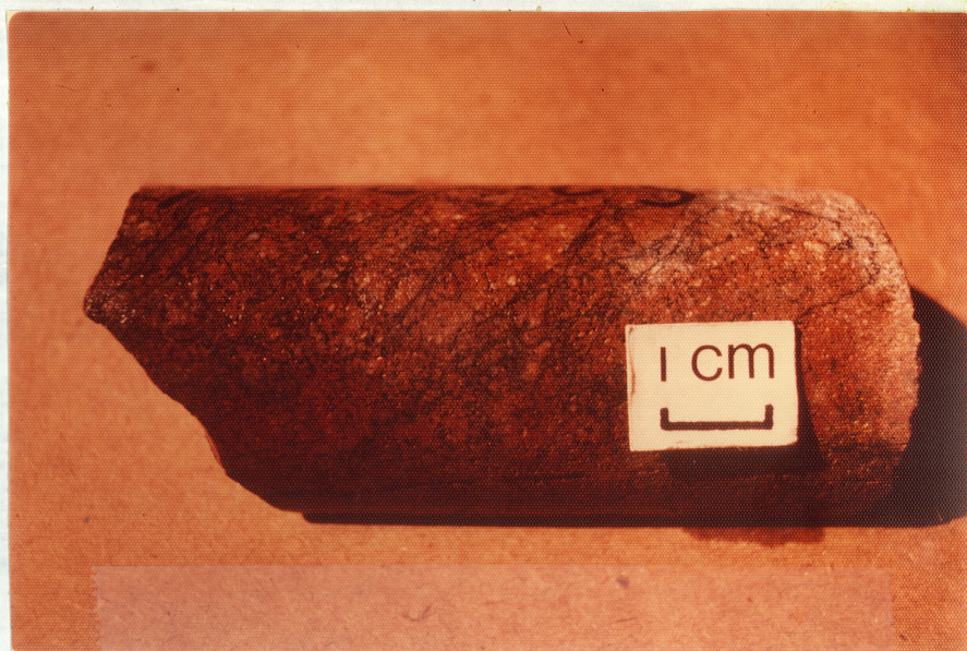
FIGURE 14. Crackle breccia superimposed on the intrusion breccia monzonite porphyry matrix. Note the "shattered" appearance of the rock. Fractures are filled with magnetite and trace chalcopyrite.
