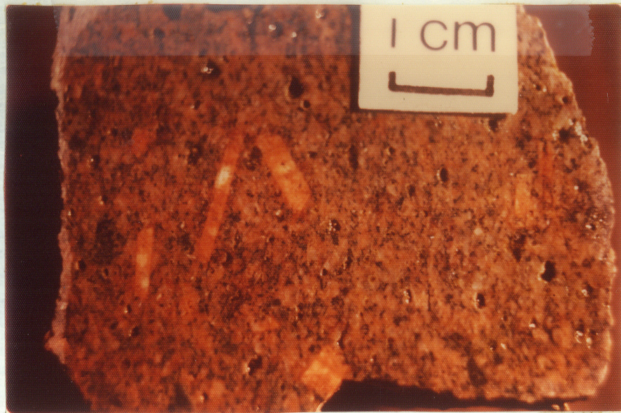
FIGURE 16. Sanidine monzonite porphyry. Note the large number of empty cavities.
