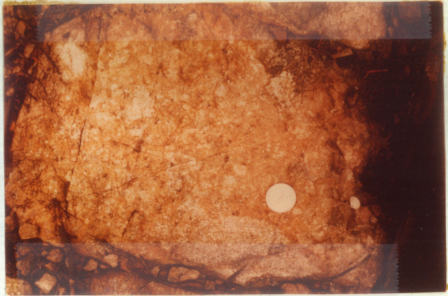
FIGURE 11. Intrusion breccia: showing syenodiorite fragment (below dime), volcanic fragment (upper right), and numerous small monzonite fragments in an altered monzonite matrix. Note subtle nature of monzonite fragments.
