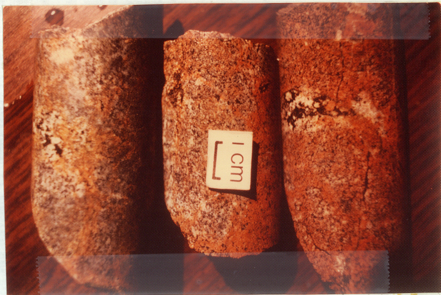
FIGURE 12. Intrusion breccia matrix showing increasing salmon pink potash feldspar alteration from left to right.
