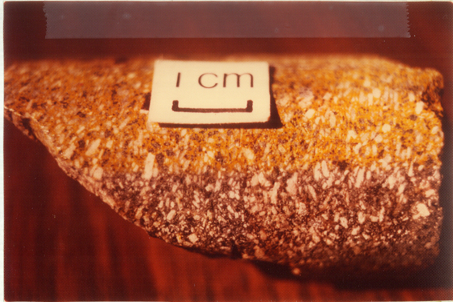
FIGURE 15. Crowded monzonite porphyry showing 50% andesine laths in an alkali feldspar matrix. Upper half of rock was stained by sodium cobaltinitrite.
