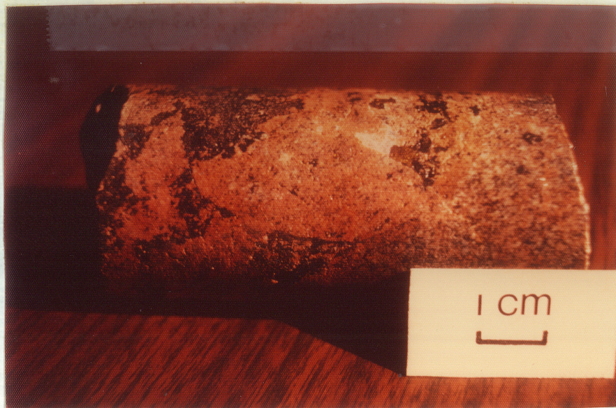
FIGURE 13. Altered monzonite porphyry fragment in monzonite porphyry matrix with irregular patches of magnetite, chalcopyrite, and carbonate.
