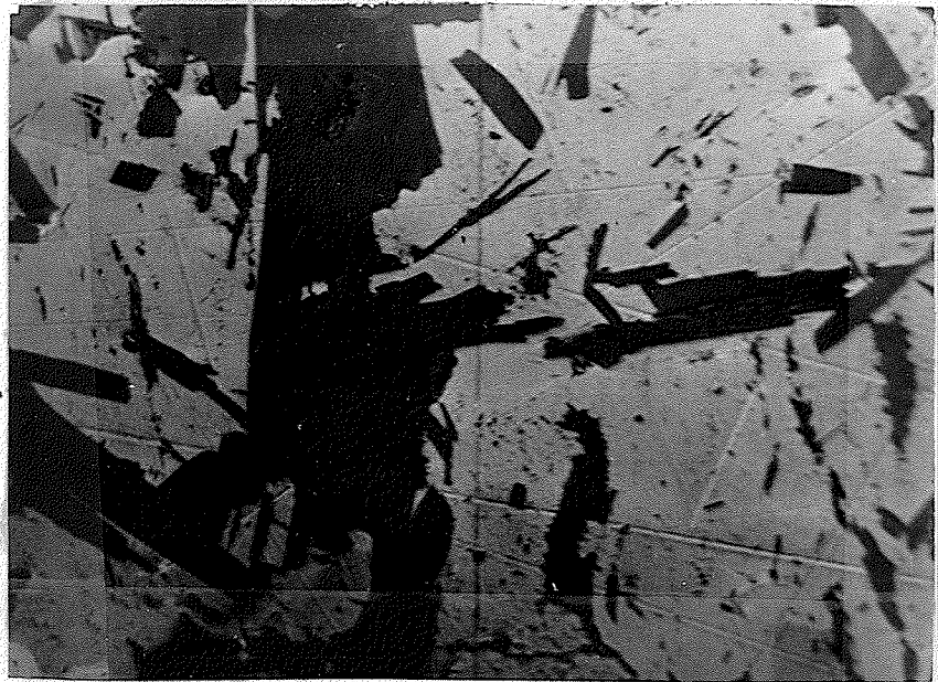
Figure 13. Disseminated sulphide ore; euhedral silicate laths within the sulphide minerals. (x 50)
