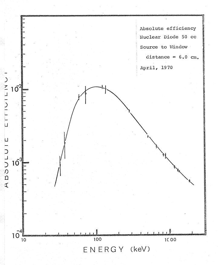
window at the source). Hence a set of calibration sources is required, and each detector has to be calibrated separately since the active volumes of two detectors are seldom, if ever, identical. The set of efficiency calibration standards issued by IEAE is shown in Table I-6. These standards are radioactive nuclides whose source strength had been carefully measured so that at any given moment, the absolute number of photons emitted can be calculated.
