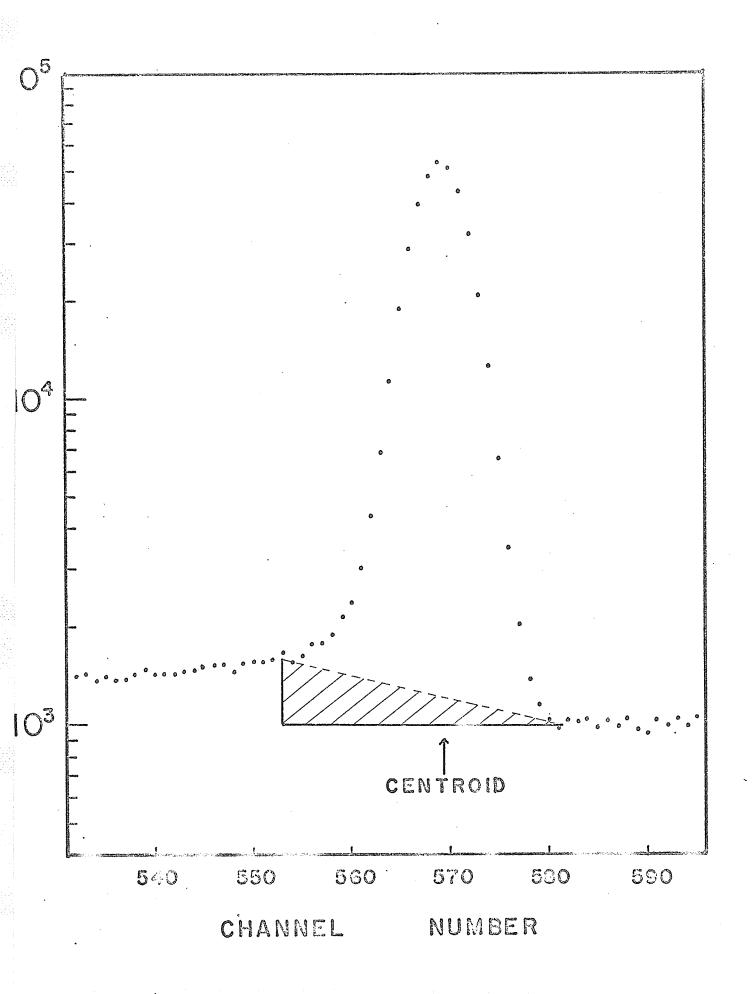
squares fitting procedure. The theory of this method is well known, and will not be elaborated here. Being of the iterative type, an initial estimate of the parameters is required to start the fitting process. The initial estimates, except the full width at half maximum (FWHM), are generated internally by the programme, and so need not be supplied but the approximate value of the FWHM must be supplied.
