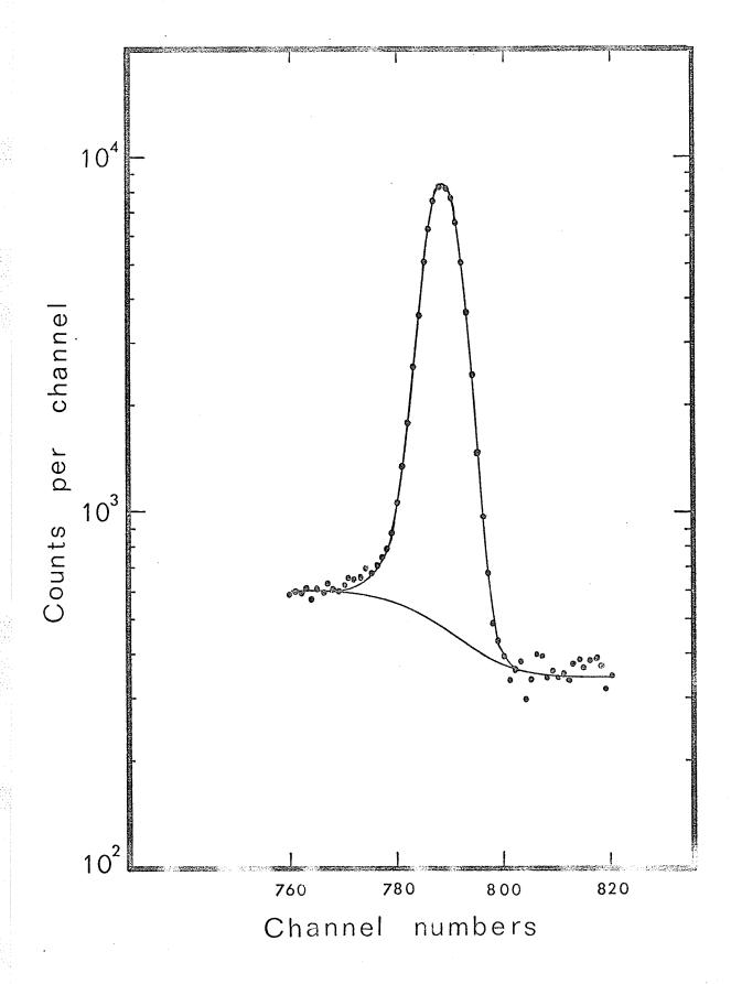
disadvantage as the previous one in that the choice of the two points is quite arbitrary, but has the advantage that when overlapping peaks are encountered, the successive stripping method can be avoided, since the one background serves for all the components.
