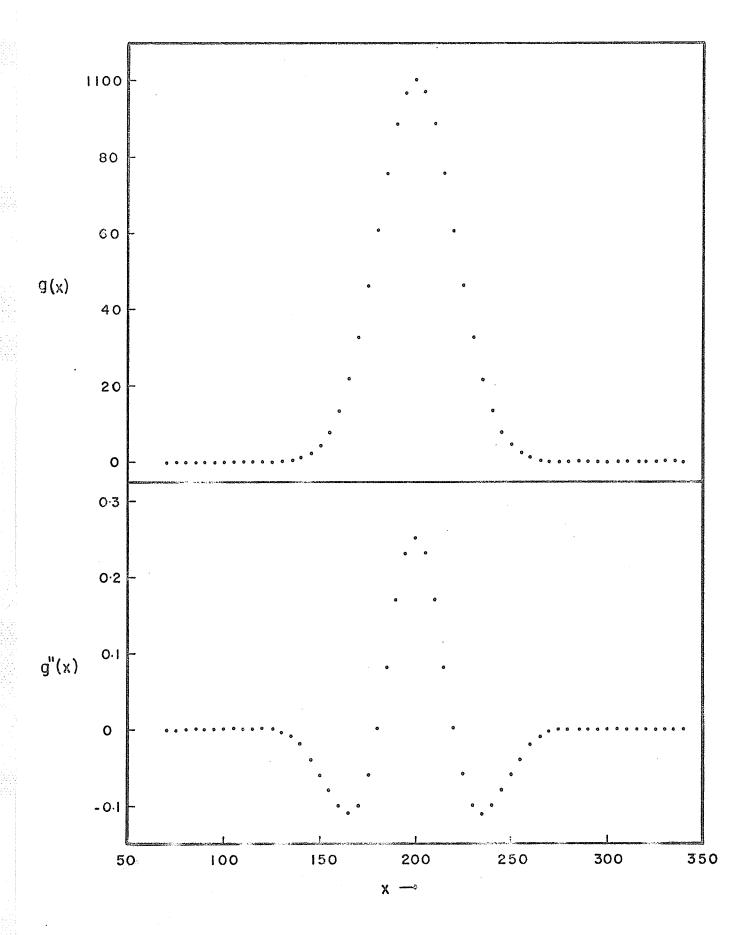
$$d = \left\{ \int_{-\sigma}^{\sigma} g''(x) x dx \right\} / \left\{ \int_{-\sigma}^{\sigma} g''(x) dx \right\}$$
