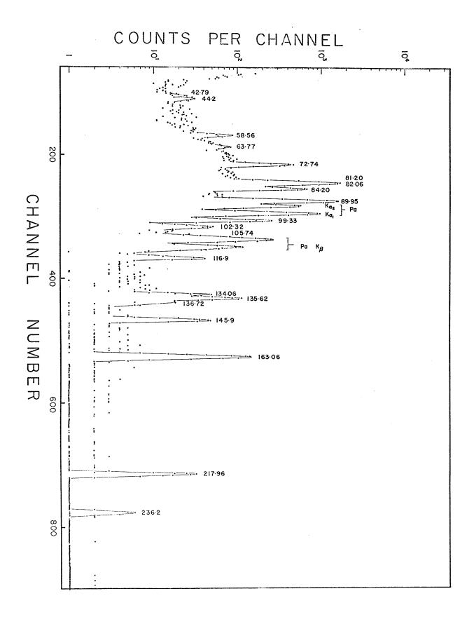
Coincidence spectrum with the 89.95 keV gamma ray
