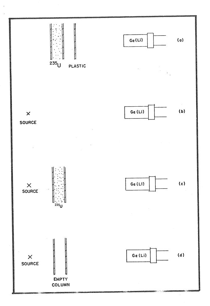
and is the quantity needed to determine the true relative intensities of the gamma rays. R is the detection rate obtained experimentally as a result of self absorption. Here a is the thickness of the resin column, and is the same as the thickness of the lucite wall.
