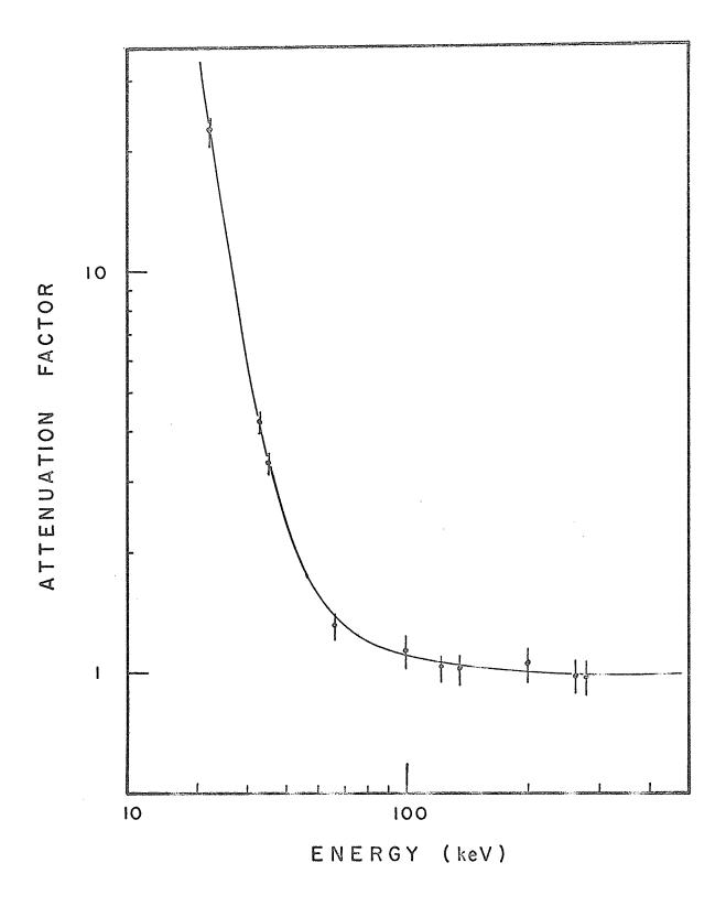
Gamma ray spectrum of 231Th decay, taken through the Mo filter
