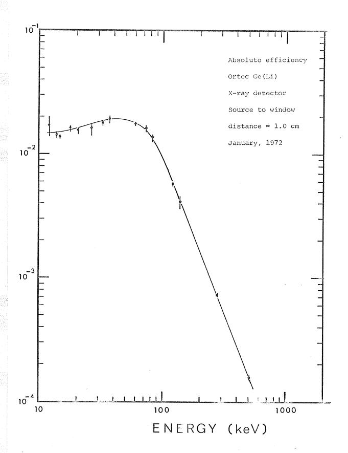
the efficiency (obtained by interpolation from the efficiency curve) at the same energy. For the sake of completeness, the efficiency curve of the Ortec Ge(Li) X-ray detector is shown in Figure I-6.
