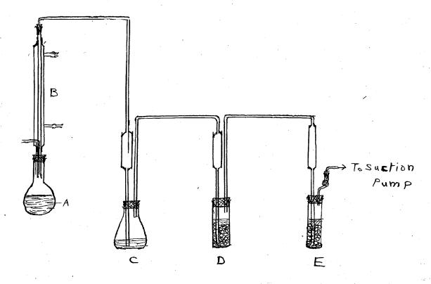
took place. To it was attached a reflux condenser B, which in turn was connected with the hydrobromic acid absorption flasks, C, D and E. C and D contained potassium iodide solution while E was filled with a known volume of standard B/2 NaOH solution. D and E were filled with glass beads. E was connected to a suction pump by means of which air was continually drawn through the apparatus during the experiment.
