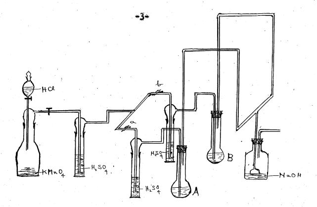
By adjusting the screw clips, a, and b, it was possible to maintain the rate of flow through each approximately equal. The flasks were removed every hour and the gain in weight noted. At the end of three hours the flasks together with their respective sulphuric acid bottles were interchanged.
