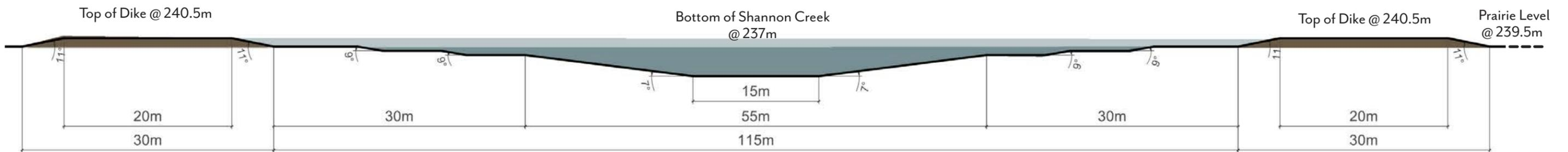
Figure 99. Condition 2 section showing high and low points. Light blue indicates seasonal water changes (Class 1-3 wetlands). Dark blue indicates Class 4 - 5 wetlands which are predicted to hold water year-round, most years.
