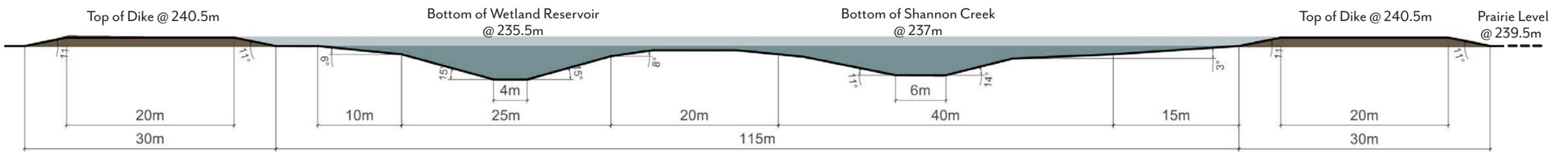
Figure 96. Condition 1 section showing high and low points. Light blue indicates seasonal water changes (Class 1-3 wetlands). Dark blue indicates Class 4 - 5 wetlands which are predicted to hold water year-round, most years.
