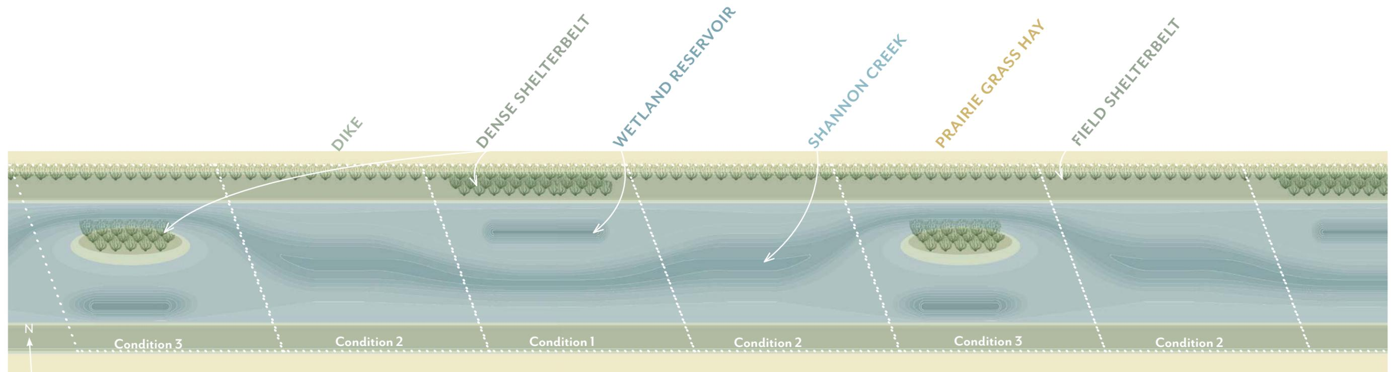
Figure 91. Channel design overview in plan perspective showing system design elements.
