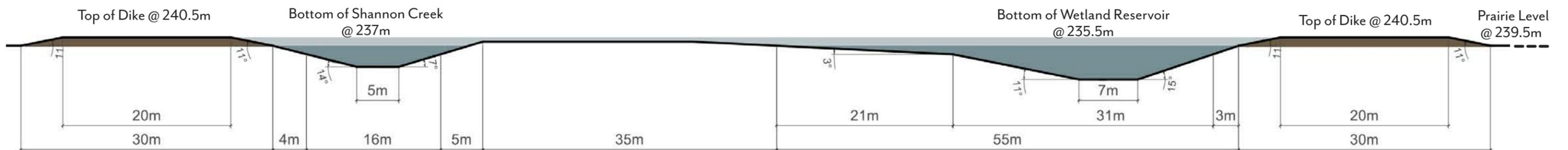
Figure 102. Condition 3 section showing high and low points. Light blue indicates seasonal water changes (Class 1-3 wetlands). Dark blue indicates Class 4 - 5 wetlands which are predicted to hold water year-round, most years.
