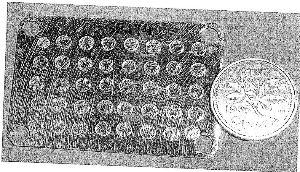
Fig. 2. The 40 spot MALDI target (1 min of HPLC elution per spot). This picture is taken from the Time-of-Flight lab in the Department of Physics and Astronomy of the University of Manitoba.
