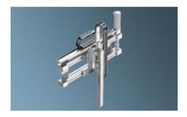
Figure 42: Linear gantry [13]. Used with Permission
