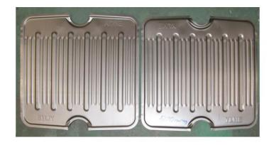
Figure 2: Individual radiator panels [2]. Used with Permission
