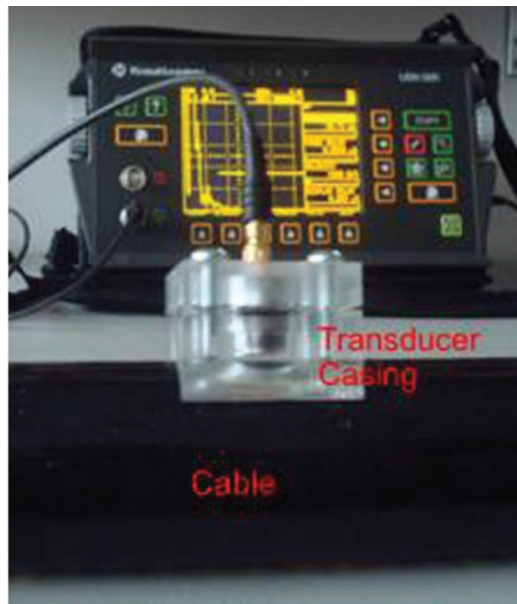
Figure 1.4: Ultrasound flaw detector, cable and casing used in [16].
