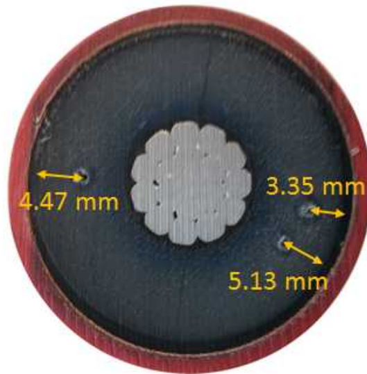
Figure 4.14: Picture of the cable under test as well as the measured sound velocities of the different layers that are on top of the XLPE insulation.
