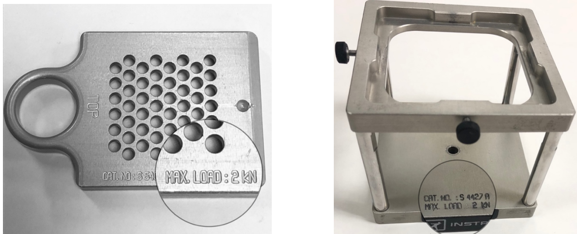
Fig. 4. 7. Extrusion insert and frame of Ottawa extrusion cell showing maximum load of 2000 N (2 KN).
