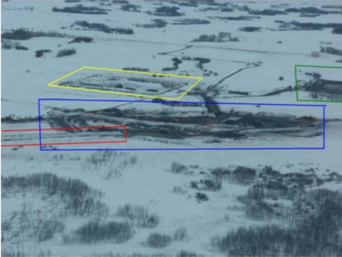
**Figure 7: Aerial Photograph of approx. 100,000 Liter Oil Spill from Broken Underground Flowline in Southwestern Manitoba near Saskatchewan Border in January 2015 - Spill is outlined in Blue (Dyck, 2015)**
