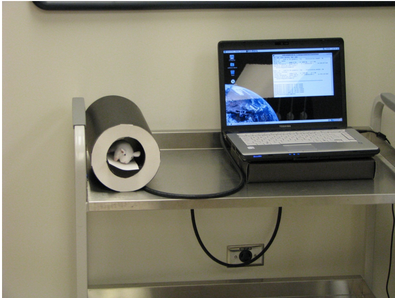
Figure 5.1 (a) Schematic of axially oriented crystal bundles (b) Photograph of a mockup of our design concept for a highly compact and portable PET imaging system.
