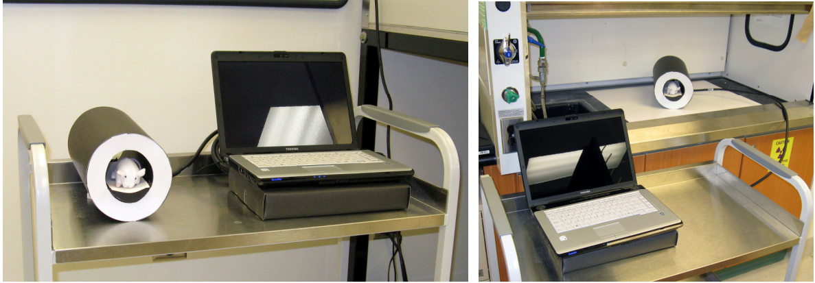
Figure 1.1 Photographs of a mock-up of our design concept for a highly compact geometry, portable PET imaging system. On the left, the system is shown on a laboratory cart. The cylindrical detector gantry has a rat sized stuffed animal in it for scale. The laptop computer for data acquisition sits on top of a compact electronics cabinet. On the right, the system is shown within a laboratory fume hood with comparable dimensions to a biosafety cabinet.
