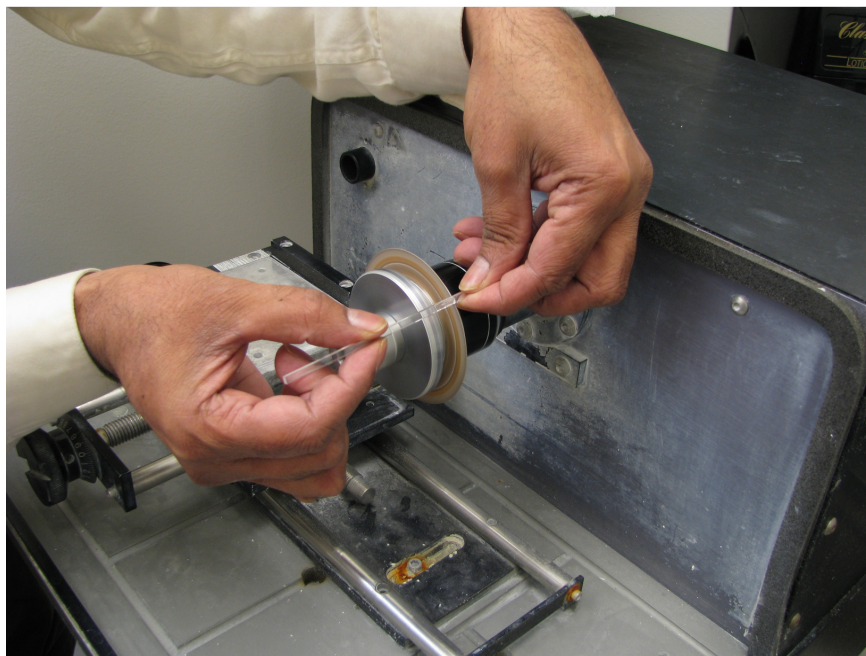
Figure 3.11 Creation of etching band patterns on a 3 × 2 × 100 mm LYSO crystal with crystal saw blade
