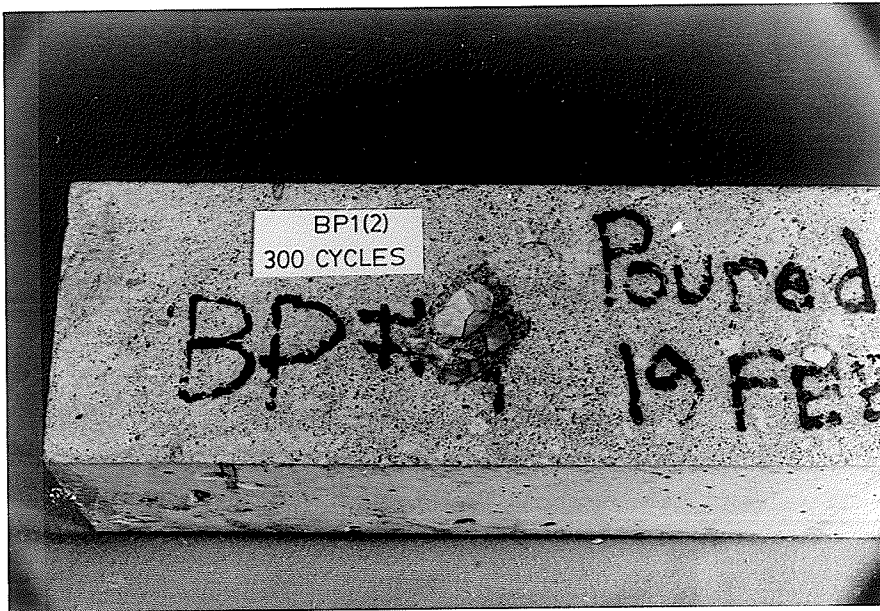
Figure 4.4: Photograph of Specimen BP1(2) After 300 Cycles of Freeze-Thaw Showing a Popout Caused by Frost Susceptible Aggregate.
