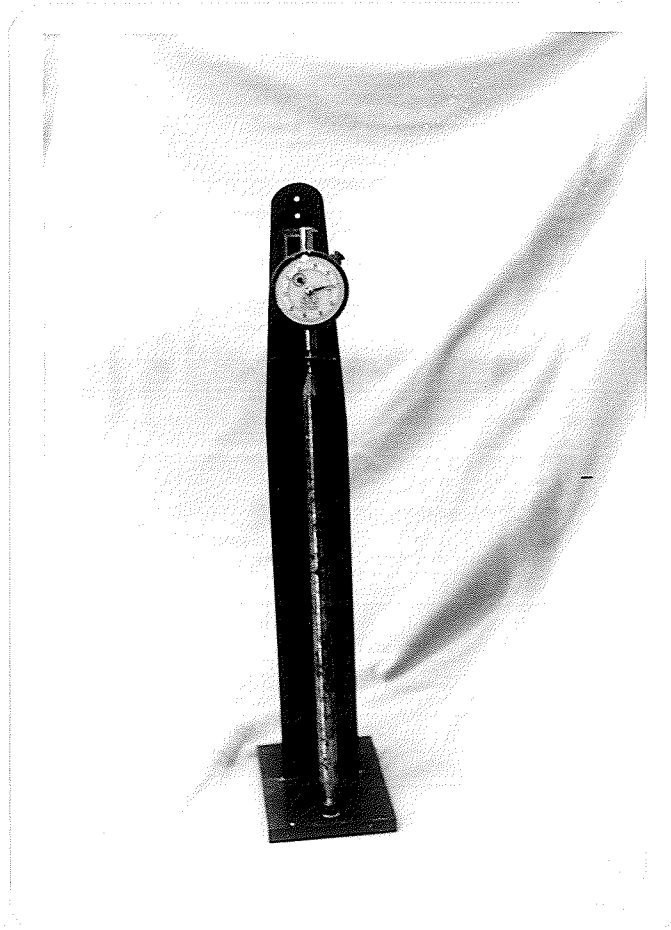
Figure 3.6: Photograph of Length Comparator Used to Determine Axial Length Changes of the Test Specimens
