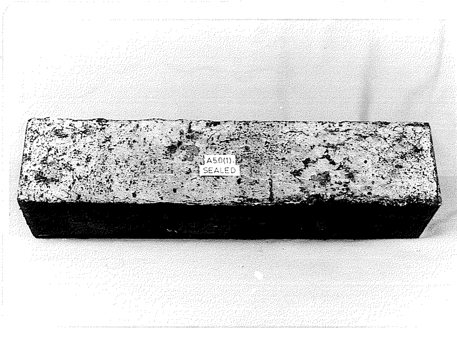
Figure 5.11: Photograph of Specimen A5.0(1) After 300 Cycles of Freeze-Thaw Exhibiting Classic D-Cracking Pattern
