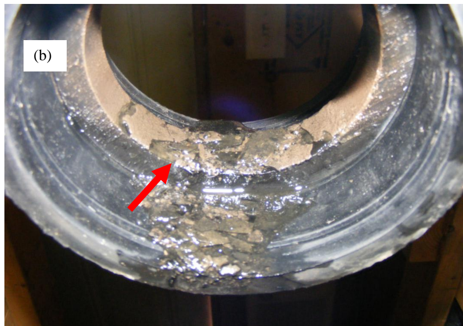
Figure 3.13. Clog development within the (a) 0.048 m and (b) 0.092 m pipes (solid arrows indicate the clog material accumulated within the pipe rings)
