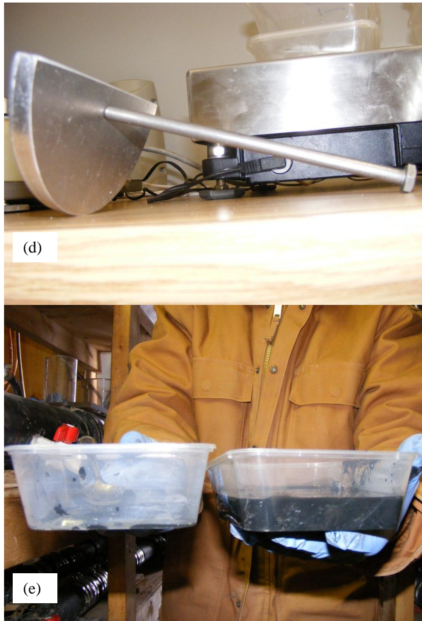
Figure (d) shows the tool built at the mechanical engineering laboratory to collect clogging from the inlet and outlet of the pipe series at 13 cm of distance inside of the pipes. Figure (e) shows how important was the difference of clogging accumulated between inlet versus outlet for the pipe series 8.
