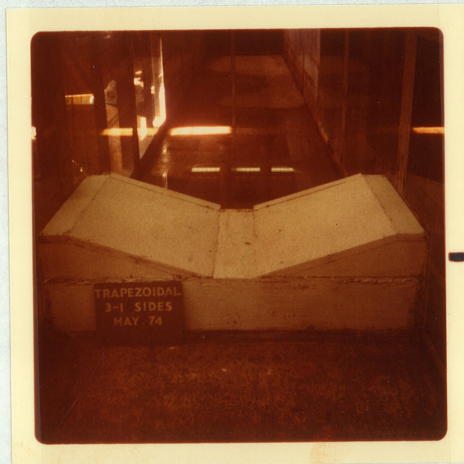
PHOTOGRAPH III-1 Typical Test Weir
