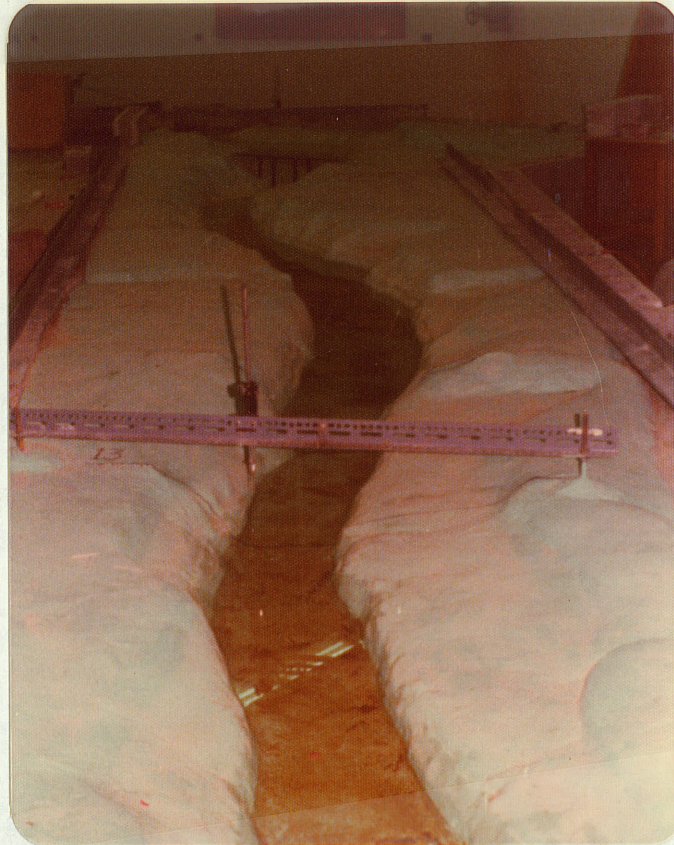
PHOTOGRAPH B3-3 Burntwood River Model Upstream of Bridge
