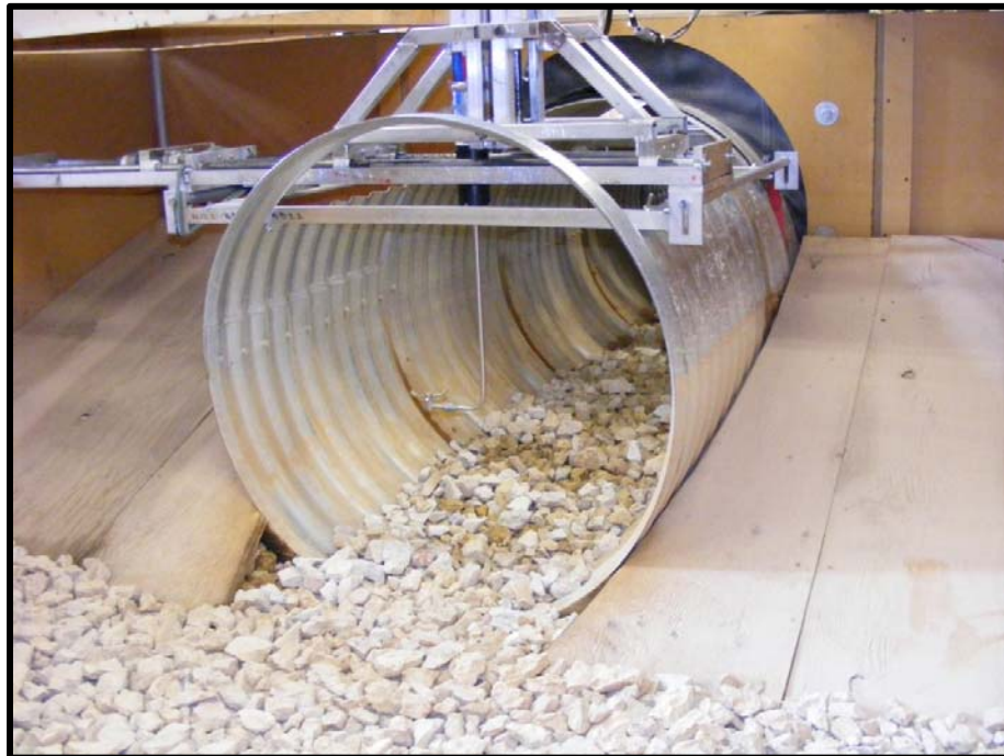
Figure 3-5: Projecting End Backfilled Inlet Configuration
