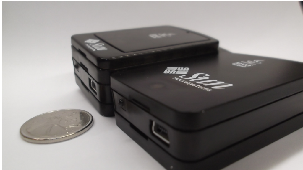
Figure 4.21: A SunSPOT free-range mote and SunSPOT base station.
