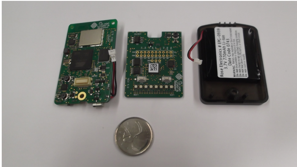
Figure 4.22: A SunSPOT taken apart to view the components in the casing.
