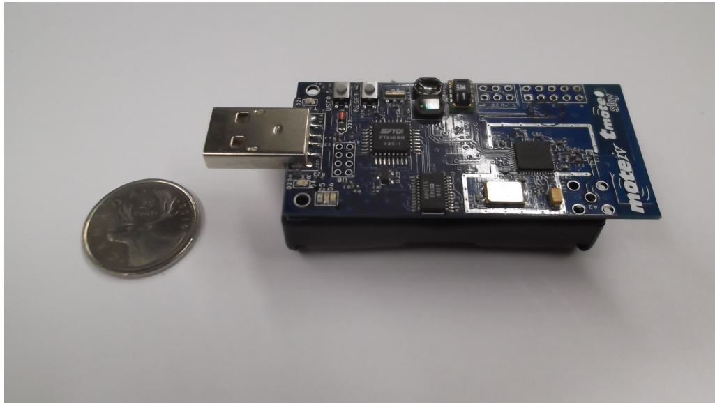
Figure 4.26: The tMote Sky, which is a Telos variant.
