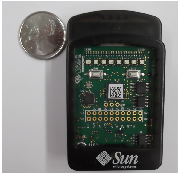
Figure 4.20: The Sun Microsystems SunSPOT.
