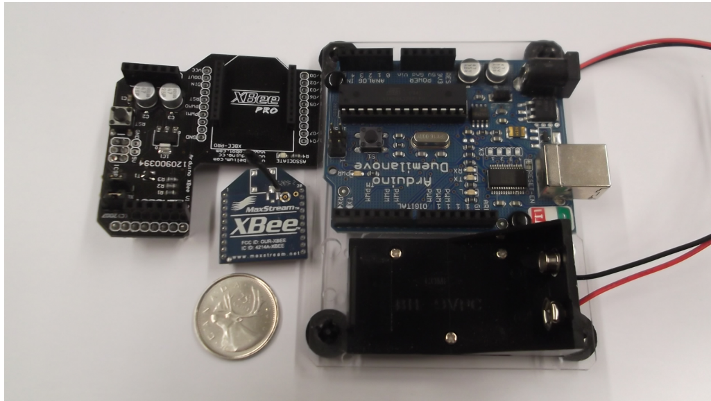
Figure 4.25: The parts used to make the Arduino mote.
