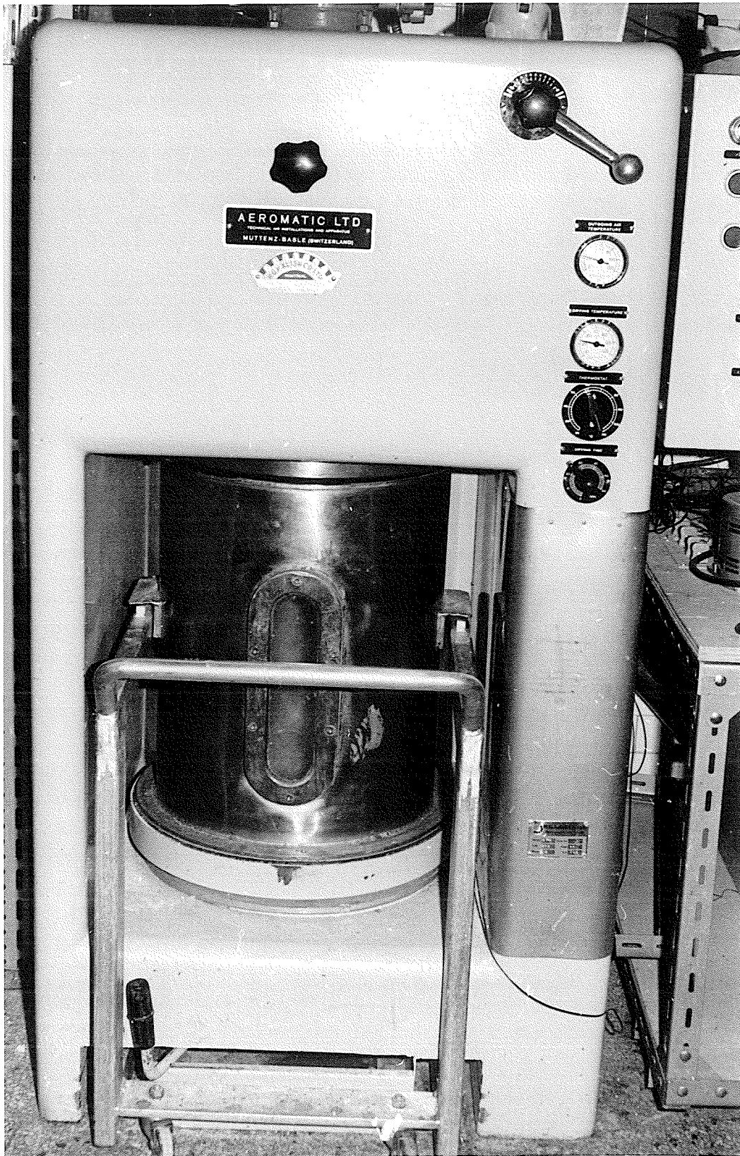
Photograph of a STS 5 Batch type fluidized bed drier
