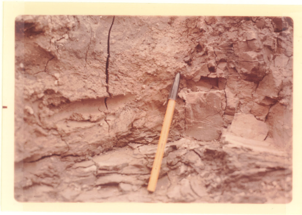
Fig. 19 Ice rafted till fragment in lacustrine clay unit. This photo taken at bottom of a 9 foot cut.
