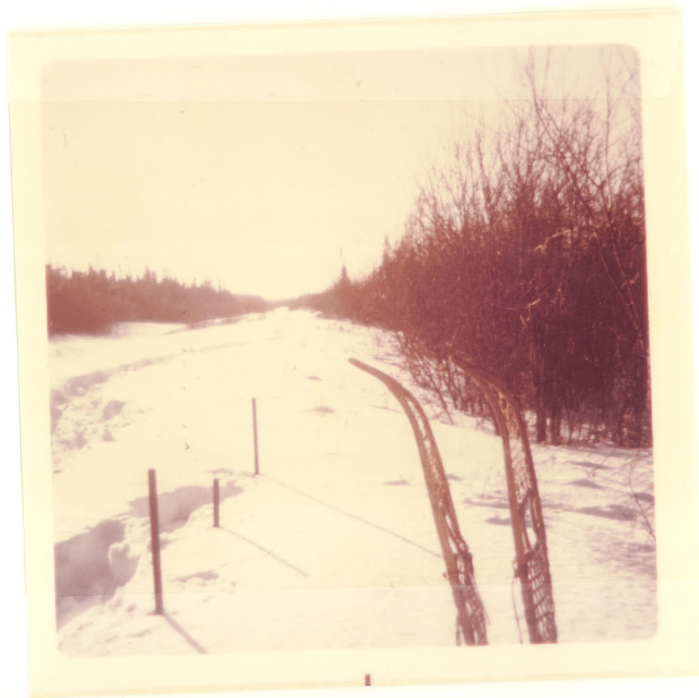
Fig. 12A Reading water levels in piezometers in late fall after water-table freezing begins.
