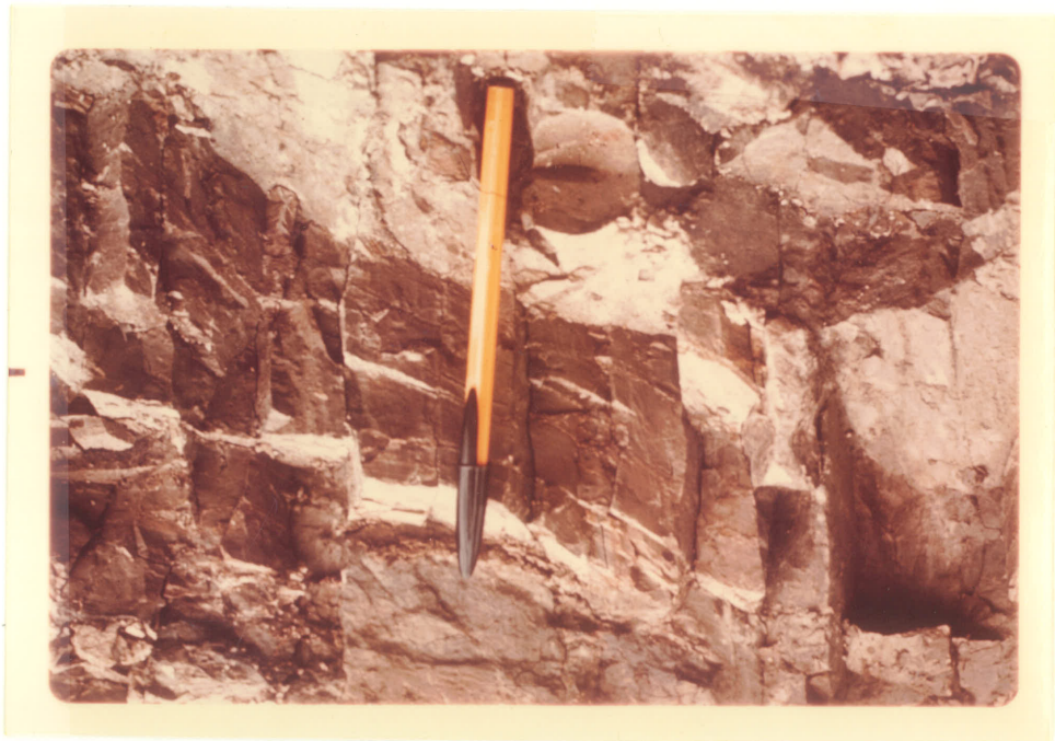
Fig. 6A Jointing in lacustrine clay unit without visible precipitates.
