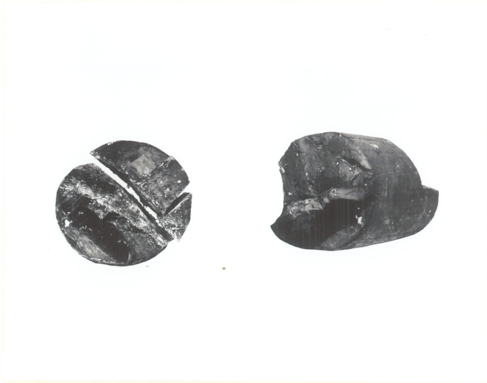
Fig. 5A Jointing in lacustrine clay unit with precipitates on joint surfaces.
