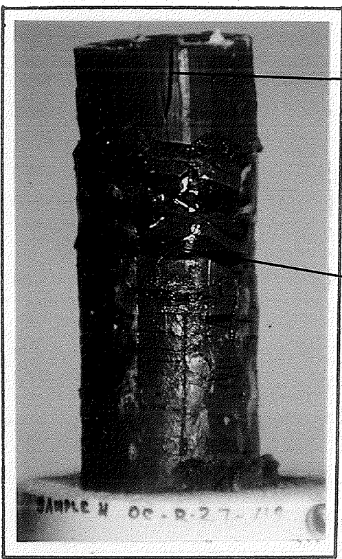
Photograph 6.6 Ice crystallization produced by external water supply during freezing process of sample OC-R-27-119
