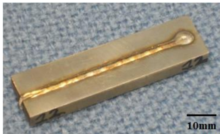
Figure 3.2: Bead-on-plate fiber laser weld of IN 718
