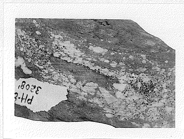
Fig. 13. Sandy band in Lower Amaranth showing the association of coarse, well rounded and frosted sand grains, rounded fragments of anhydrite, and angular fragments of dolomite. The band shows considerable inclination to the core. Pascas Hunt 10-9-1-27 well at 3208 feet. (X 1)
