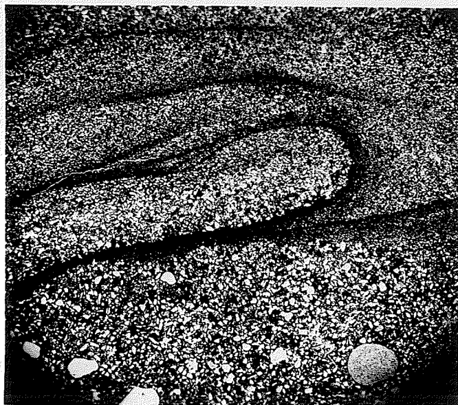
Fig. 18. Lower Amaranth siltstone showing pronounced slumping or flowage structure. The dark laminations are argillaceous material. Note the variation in grain size from fine silt to medium sand. Grain in bottom right is weathered feldspar. Calstan Waskada 9-13-1-26. (X 15, plain light)
