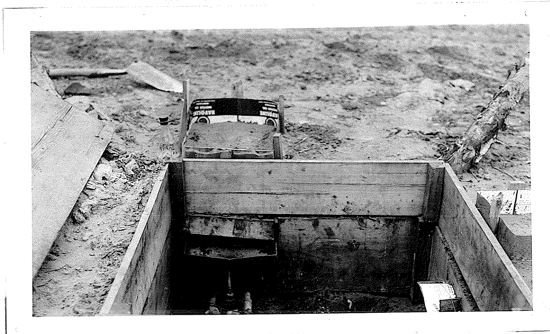
Figure No. 25 - View of Leachate "Catchment" installation in a fallow field. Note: the tin enclosures at the soil surface, the metal pans directly below, and the winchester flasks to catch the leachate running from the pans.
