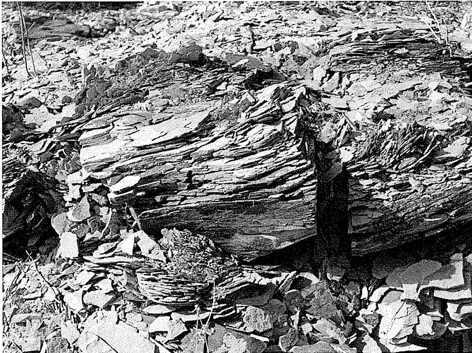
Figure 4.7 – Site 3 or PR259 and Assiniboine River, close up of the platy Millwood clay shale structure
