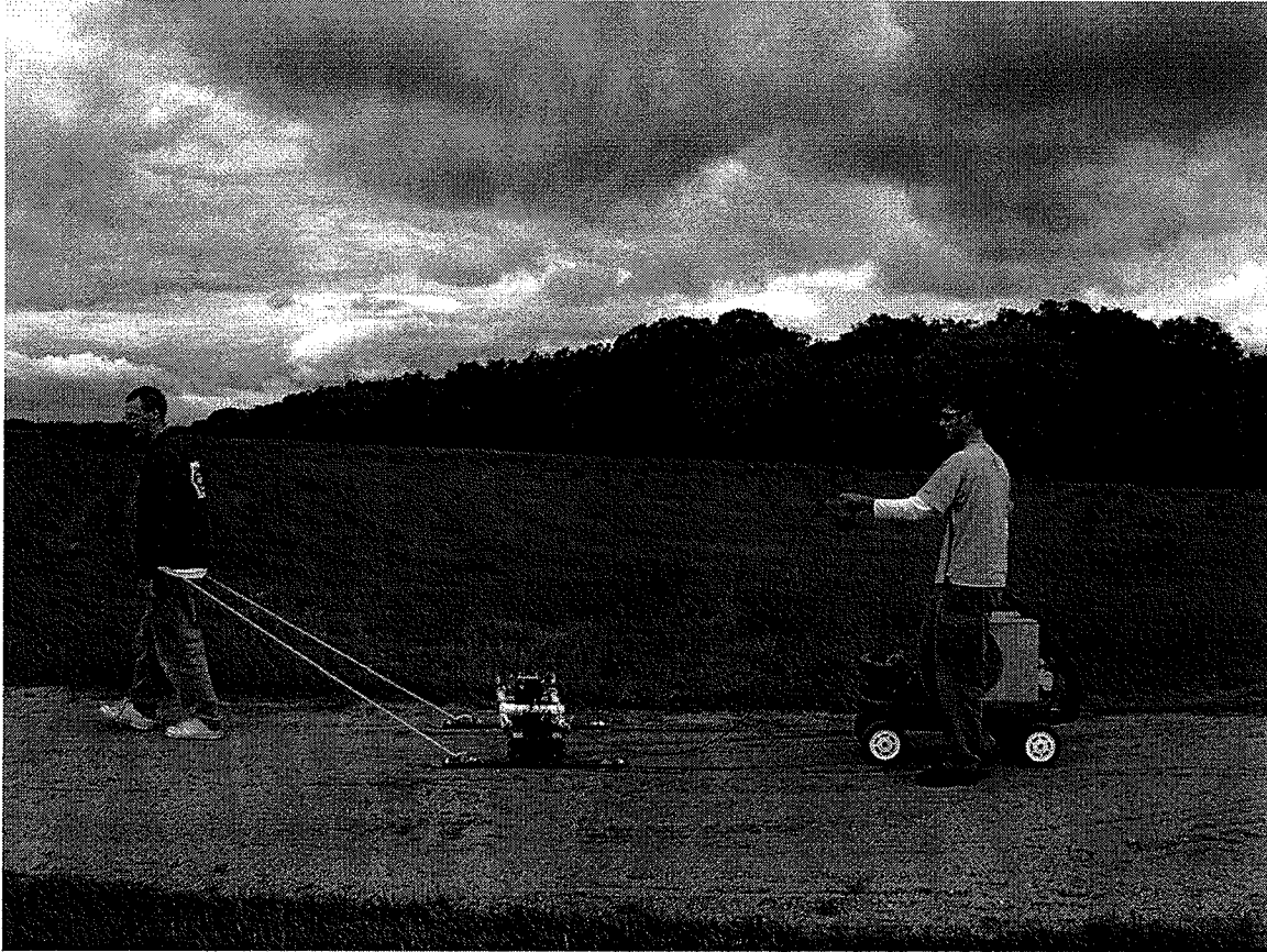
Figure 6-3. The Pulse Ekko 100 MHz GPR system in use at the Paul's Road site.
