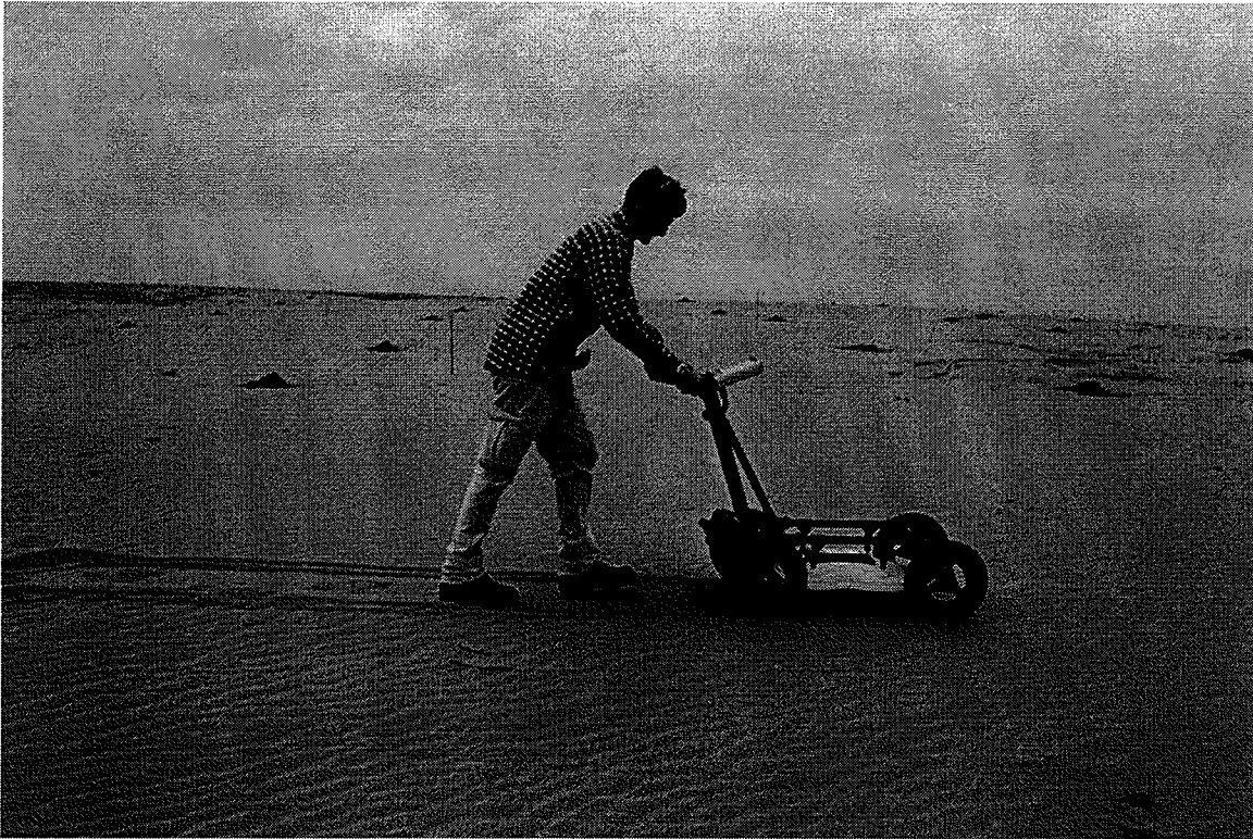
Figure 6-4. The Noggin 250 MHz GPR system in use in SW Saskatchewan (C. Hugenoltz, pers. comm., 2005).
