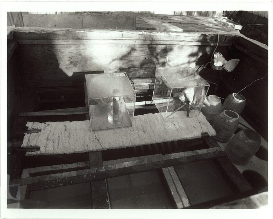
Figure 3. Waterbath used to rear *Cx. tarsalis* at 19°C and natural daylength in 1992, and *Cs. inornata* at 16°C and natural daylength in 1993. Wooden frame covered with black polypropylene (foreground) was used to shield the bath from direct sunlight.
