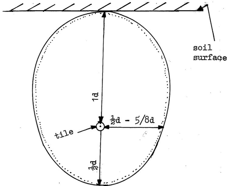
FIGURE 2-1. Cross Section View of Steam Expansion
