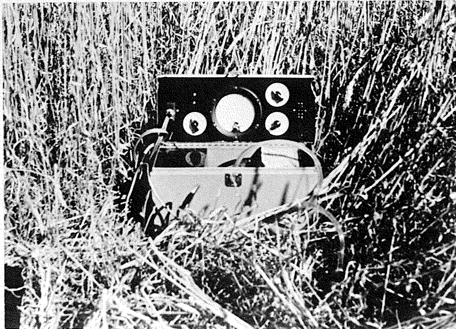
Fig. 4b Field use of the oxygen diffusion rate measuring apparatus.
