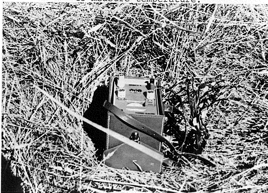
Fig. 7 Potentiometer used with thermocouples to measure temperature.
