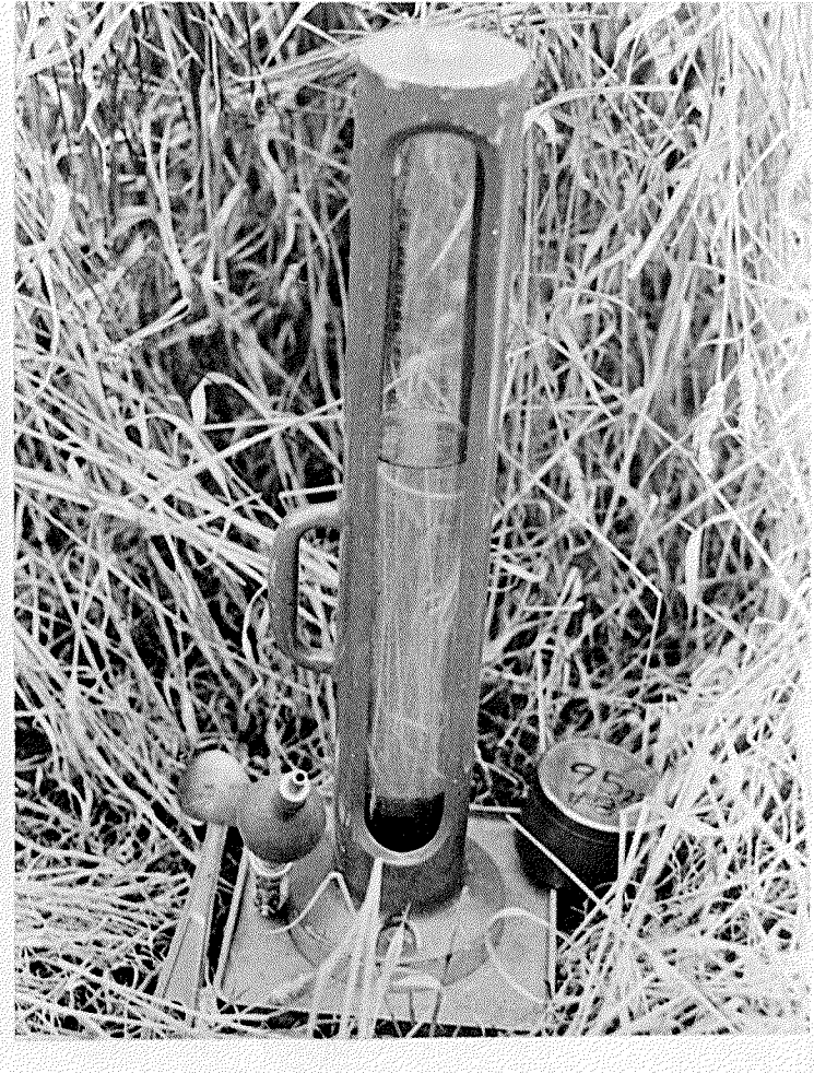
Fig. 5b Field use of the soil bulk density measuring apparatus (water balloon method).
