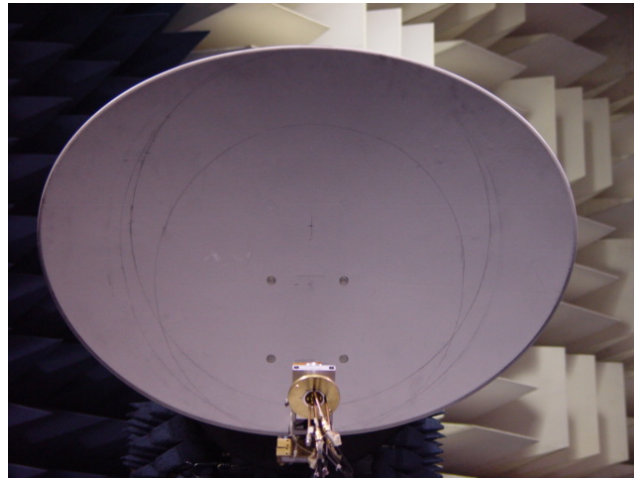
Fig. 5.18. Photograph of the prototype offset reflector antenna with the proposed feed.
