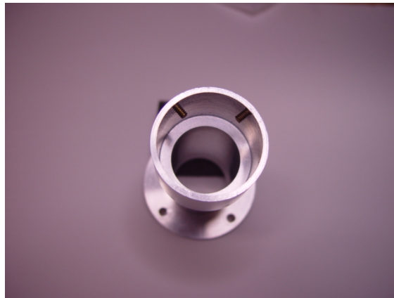
Fig. 3.25. Photograph of the prototype feed #2 (stepped waveguide with two tuning screws).
