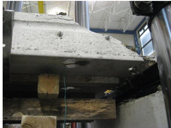
Photos of HC 200-P2-B (Web-Shear Failure)
