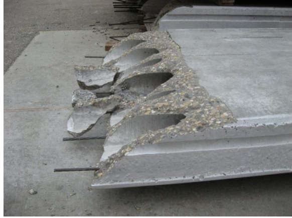
Photos of HC 200-P2A (Web-Shear Failure)
