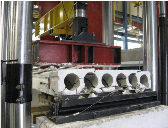
Photos of HC 200-P2-B (Web-Shear Failure)
