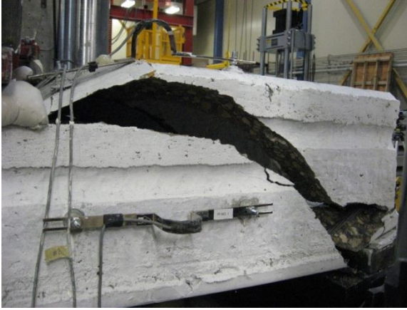
Photos of HC 200-P2A (Web-Shear Failure)
