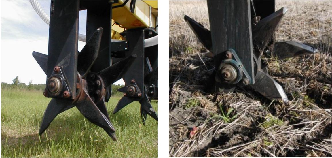
Figure 11: AerWay shatter tines; (a) mounted on the tractor toolbar; (b) pair of shatter tines penetrating into soil during a field operation
