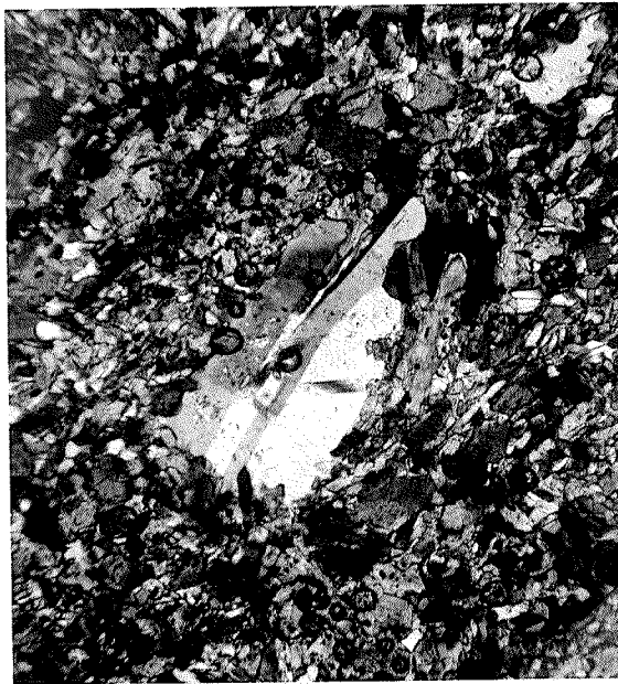
Figs. 23, 24, & 25 Primary plagioclase X 80 Primary plagioclase, plus recrystallized plagioclase and hornblende.
