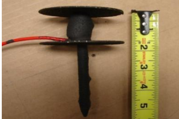
Figure A-23 Vertical Asphalt Strain Gauge.
