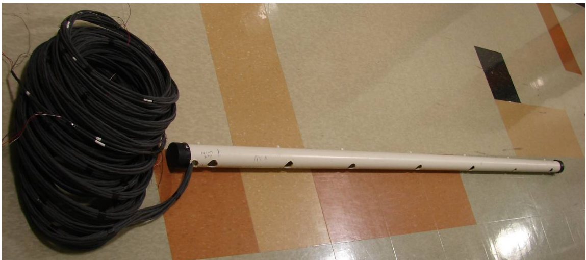
Figure A-19 Thermistor string with seven thermistor probes.
