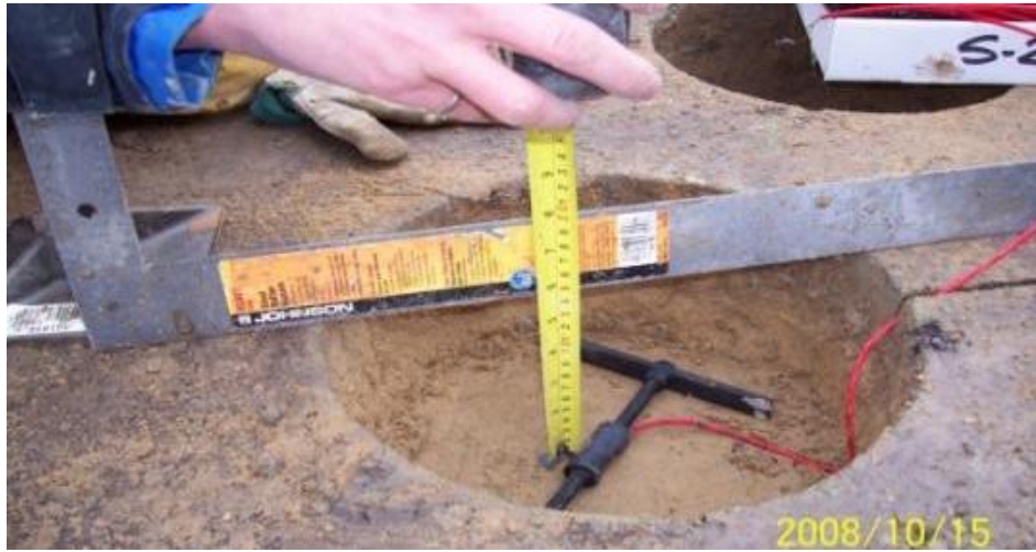
Figure A-26 Installing horizontal ASG at PR304.
