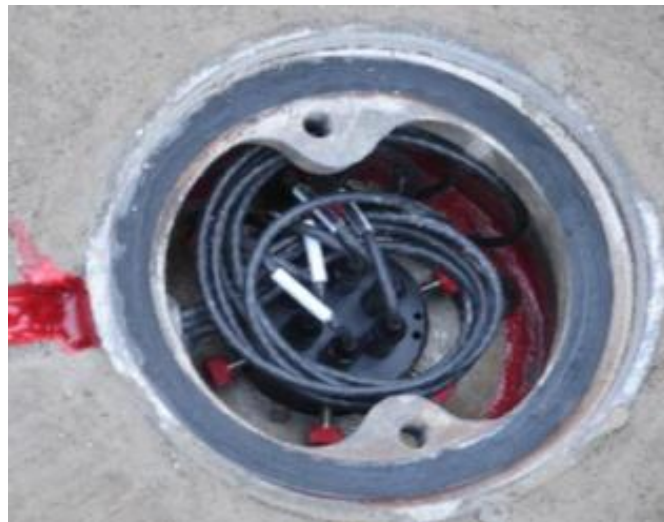
Figure A-43 Six transducers inserted in the reference head within MDD road box.
