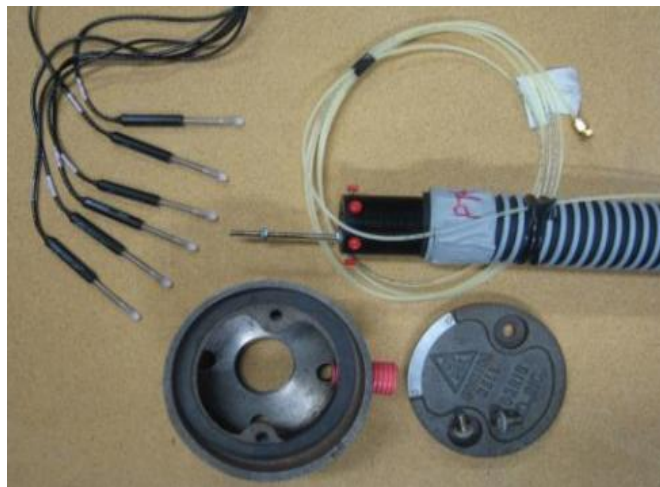
Figure A-380 Reference head, road box, and transducers of MDD.
