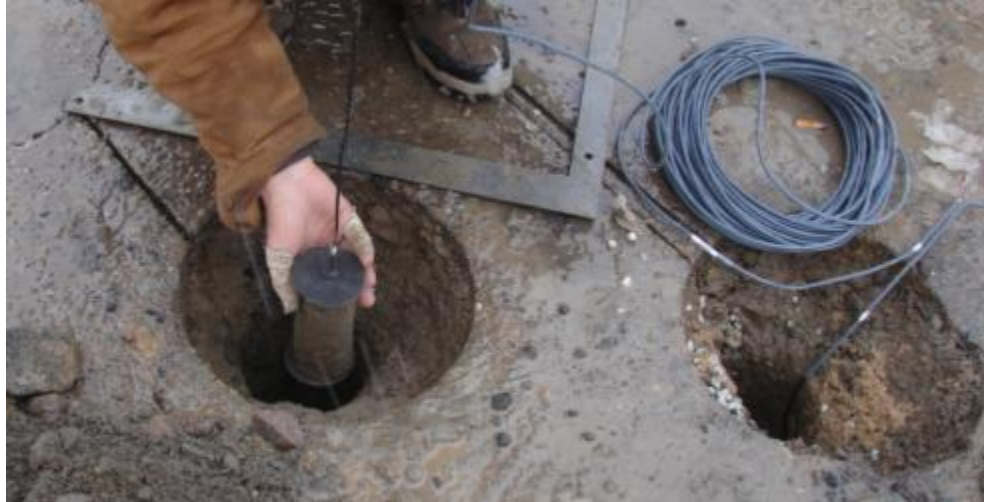
Figure A-36 Insert the mass of soil and SCG into hole at PR304.
