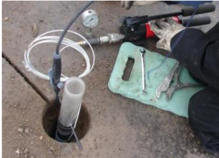
Figure A-40 Expansion of the MDD hydraulic anchor.
