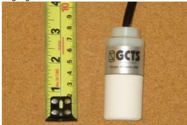
Figure A-12 Fredlund Thermal Conductivity sensor (FTC-100).
