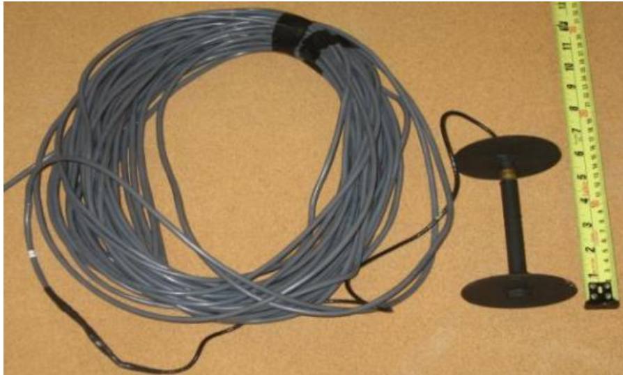
Figure A-32 Soil compression gauge.
