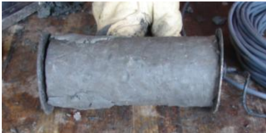
Figure A-35 Pack the two halves of soil mass around SCG.
