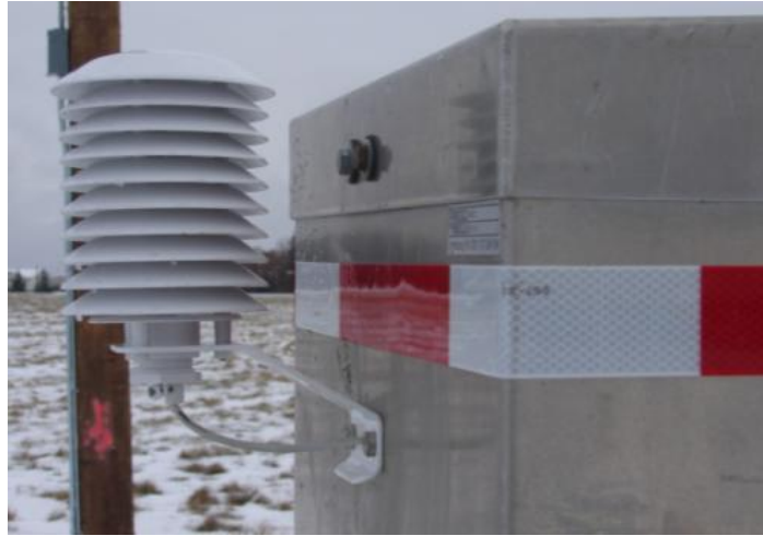
Figure A-21 Humidity and temperature probe beside a DAS
