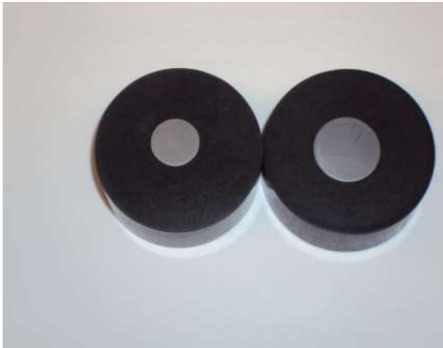
Figure 3.9: Impacted AISI 4340 Steel Samples Mounted in Bakelite
