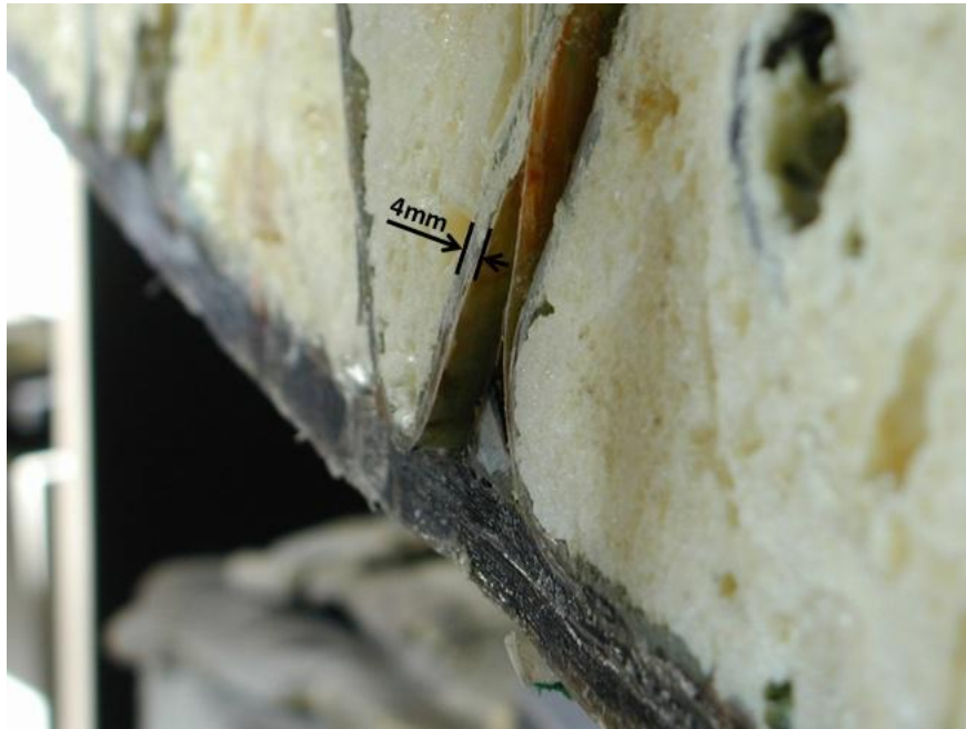
Figure 3.10: Slippage of a triangular inside tube (adapted from Williams, 2000b)
