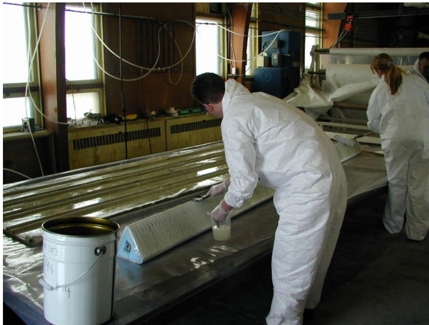
Figure 4.42: Spreading epoxy resin on a triangular inside tube (Crocker, 2001)
