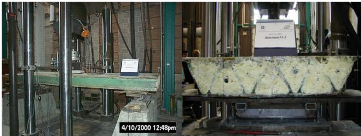
Figure 3.6: Test setup of the second-generation GFRP bridge deck (Williams, 2000b)
