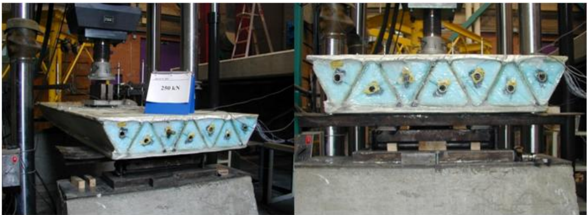
Figure 3.8: Test setup of the fourth-generation GFRP bridge deck (Crocker, 2001)
