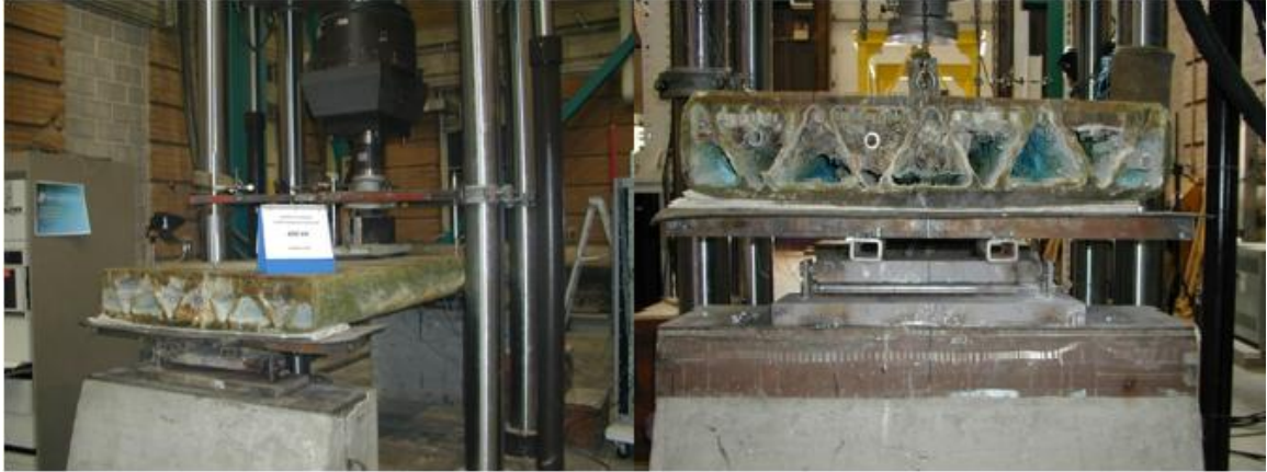
Figure 3.7: Test setup of the third-generation GFRP bridge deck (Crocker, 2000)
