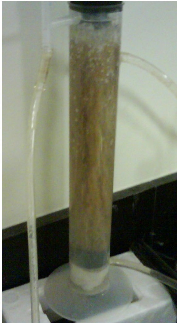
Figure 5.4 Pictures of the nitrification reactor (PMP)
