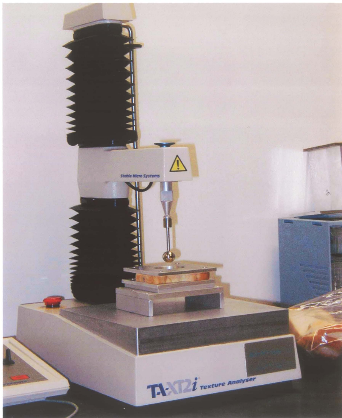
Figure 6. TAxT2 Texture Analyser and Bread Holding Apparatus.
