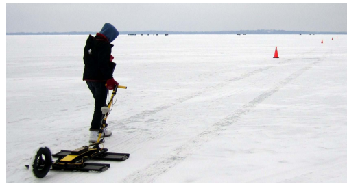
Figure 1.2: Measuring ice thickness for roads [9].
