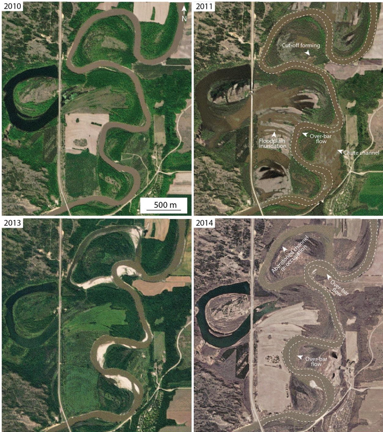
Fig 2.14. Satellite images of the Assiniboine River during annual flows (2010, 2013) and during extreme floods (2011, 2014). The channel during annual flow is superimposed on the river during extreme flooding to highlight the differences. The formation of a cut-off, floodplain inundation, over-bar flow, and the WRPB chute channel are indicated on the 2011 satellite image. The re-occupation of the abandoned channel and over-bar flow are indicated on the 2014 satellite image. Satellite images courtesy of Planet Labs.
