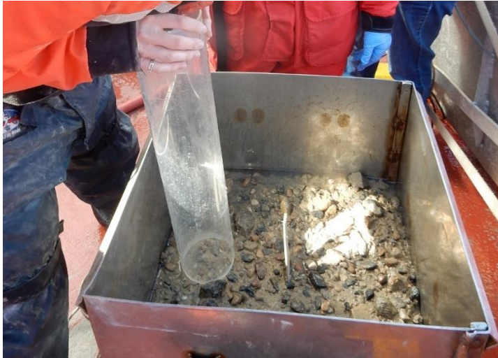
Figure 4-8: Photo of the coarse-grained materials at the surface of core 32.
