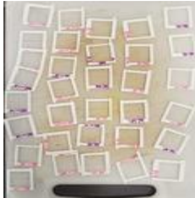
Figure 2.3. Fibres Attached to the Frames by Glue
