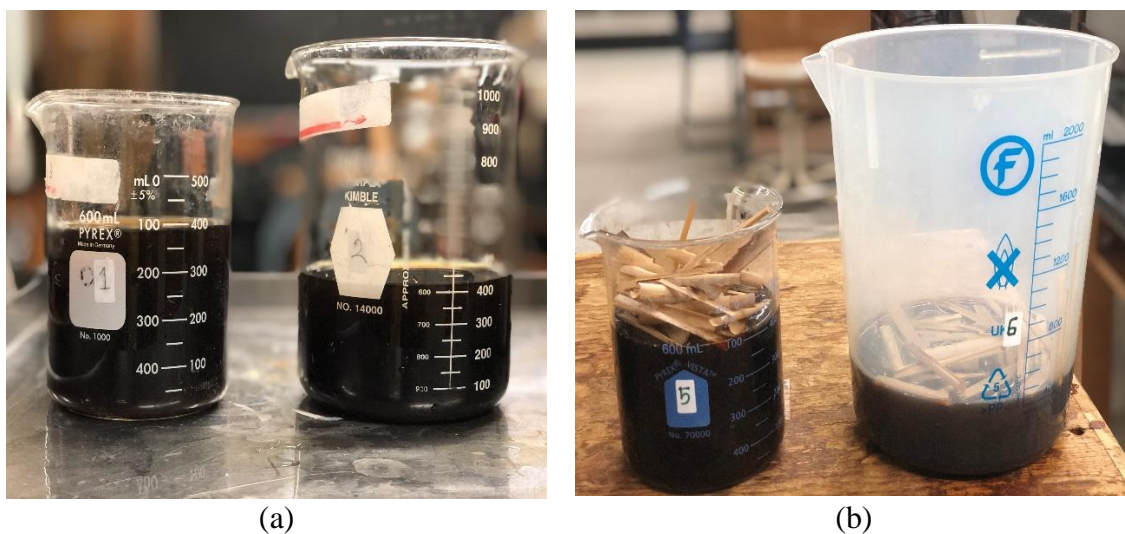
Figure 2.7. a. Third time after Reuse NaOH Alkali Solution; b. 17th time after Reuse NaOH Alkali Solution.
