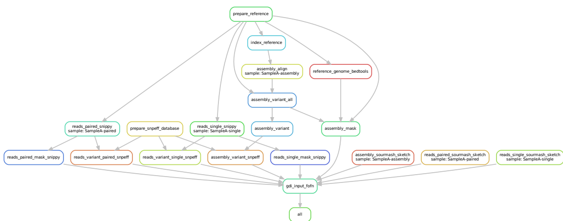
Figure A.1: A Directed Acyclic Graph (DAG) of the GDI analysis pipeline on three different samples: SampleA-single , SampleA-paired , and SampleA-assembly . This shows the dependencies among different stages of the analysis pipeline, which is used by Snakemake [90] to schedule jobs either sequentially (those stages on the same path in the graph) or in parallel (those stages on parallel paths in the graph). The final stage gdi_input_fofn is used to gather all the required files by GDI for the indexing stage ( i.e. , VCF, BED, and sourmash sketches) into a single tab-delimited file of file-paths. This figure was constructed using the snakemake --dag | dot -Tpdf command as described in the Snake- make documentation.
