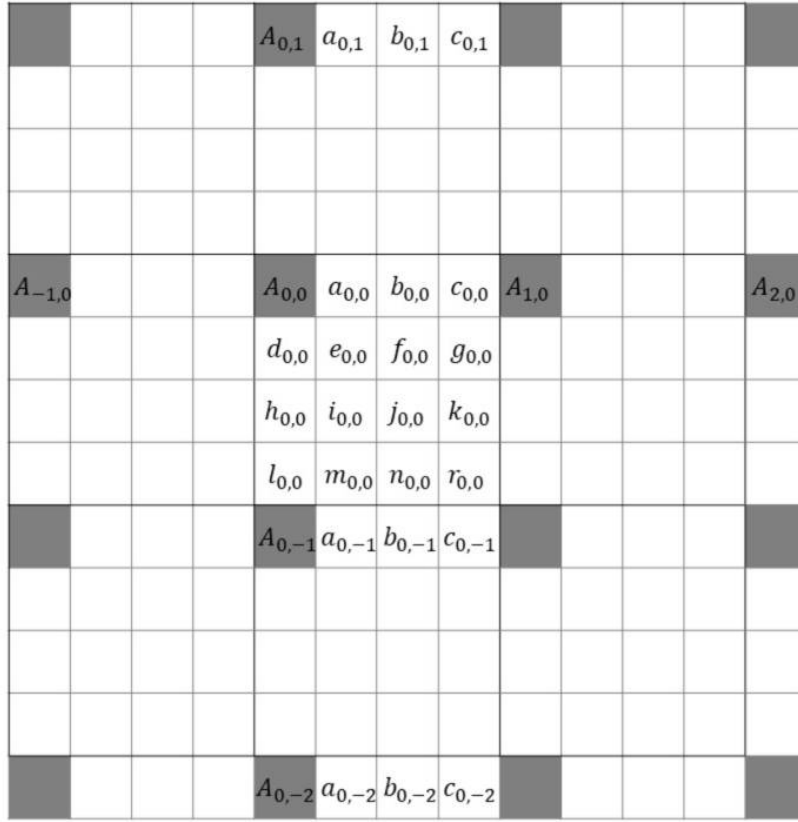
FIG. 4.7: Integer pixels (shaded blocks with upper-case letters) and fractional-pixels (un-shaded blocks with lower-case letters) for quarter-pixel interpolation.
